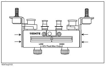
**Step 1.** Set the 16047E test fixture to the UNKNOWN connectors on the instrument by gradually coupling the four BNC connectors and fastening screws of the fixture with the connectors of the instrument until they come to complete contact. Be sure to align the grooves on both sides.
