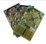
This is a small demo board with a PIC18F45K20 device on board and a small, surface-mount prototype area. Use it with a PICkit 3 In-Circuit Debugger to program your code via a 6-pin ICSP header on the board. This product also includes two bare PCB boards for those interested in customizing their development. This 44-Pin Demo Board also comes bundled with the PICkit 3 Debug Express if you order the DV164131.
