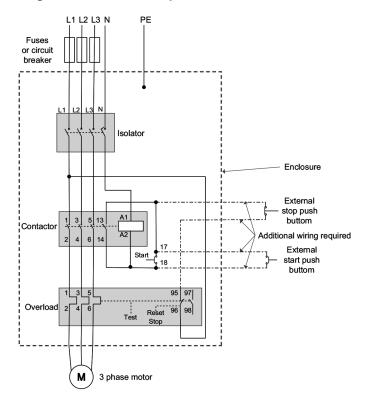
Additional start and stop stations can be wired to the DOL control circuit. In principle, the start buttons should be momentary normally open device and wired in parallel with terminals 17 & 18.
