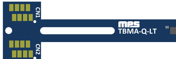
Figure 1: TBMA Test Boards
