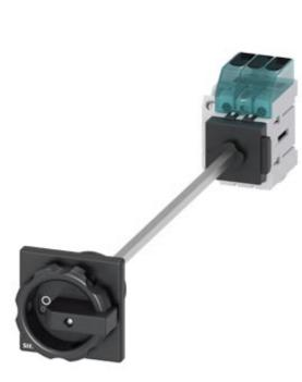
Switch disconnector 3LD3, main switch 3-polig, lu 32A operational switch at AC-23 A at 400 V 11,5 kW floor mounting Base mounting with door coupling center-hole 22,5 mm rotary operationg mechanism black 66 x66 mm with auxiliary 1NO+1NC
