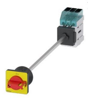
Switch disconnector 3LD3, main switch 3-polig, Iu 40A operational switch at AC-23 A at 400 V 15,0 kW floor mounting Base mounting with door coupling center-hole 22,5 mm knob-operated mechanism red/yellow  $48 \times 48 \text{ mm}$
