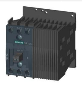
SOLID-STATE CONTACTOR 3-PH 3RF3 AC53 9.2A 40 DEGREES C 48-600V / 110-230V AC 2-PH. CONTROLLED INSTANTANEOUS SCREW TERMINALS
