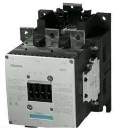
CONTACTOR, 160KW/400V/AC-3 WITHOUT COIL AUXILIARY CONTACTS 2NO+2NC 3-POLE, SIZE S10 MAIN COND.: BAR CONNECTIONS CONVENT. OPERATING MECHANISM AUX. COND.: SCREW TERMINALS
