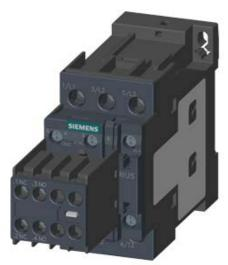
CONTACTOR, AC-3, 5.5KW/400V, 2NO+2NC, DC 220V, 3-POLE, SZ S0 SCREW TERMINAL REMOVABLE AUX. SWITCH
