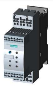
SIRIUS SOFT STARTER, S0, 32A, 18.5KW/500V, 40 DEGR., AC 400-600V, AC/DC 24V, SPRING-LOADED TERMINALS
