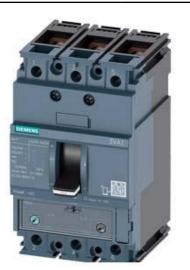
CIRCUIT BREAKER 3VA1 IEC FRAME 160 BREAKING CAPACITY CLASS N ICU=25KA @ 415 V 3-POLE, LINE PROTECTION TM240, ATAM, IN=160A OVERLOAD PROTECTION IR=112A ...160A SHORT CIRCUIT PROTECTION II=5...10 X IN BUSBAR CONNECTION
