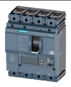
CIRCUIT BREAKER 3VA2 IEC FRAME 160 BREAKING CAPACITY CLASS C ICU=110KA @ 415 V 4POLE, LINE PROTECTION ETU860, LSIG, IN=160A OVERLOAD PROTECTION IR=64A ...160A SHORT CIRCUIT PROTECTION ISD=0,6..10X IN, II=1,5..10X IN NEUTRAL PROTECTION ADJUSTABLE (OFF, UPTO 100%) GROUNDFAULT, SWITCHABLE IG=0,2... 1 X IN, TG=0,050,8MS CABLE CONNECTION
