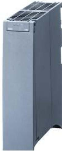
SIPLUS S7-1500 CM PTP RS422/485 -40 ... +70 GRAD C MIT CONFORMASL COATING BASED ON 6ES7541-1AB00-0AB0 . KOMMUNIKATIONSMODUL FUER SERIELLE VERBINDUNG RS422 UND RS485, FREEPORT, 3964(R), USS, MODBUS RTU MASTER, SLAVE, 115200 KBIT/S, 15-PIN SUB-D BUCHSE
