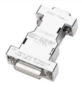
RS422 TO TTY CONVERTER, MALE (9-PIN) TO FEMALE (15-PIN), FOR SCREW CONNECTION TO RS 422 INTERFACE, 180 DGR CABLE OUTLET, FOR CONNECTION OF SIMATIC S5
