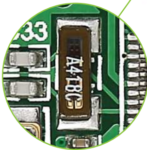
Figure 6-1: 32.768 kHz crystal oscillator module (X2)
