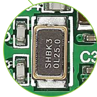
Figure 6-2: 25MHz crystal oscillator module (X1)
