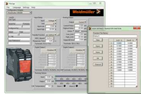
example of user defined transfer function for assigning customized output values
