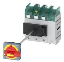
SENTRON, Molded case switch 3LD5 UL, Emergency switching-off, 4-pole, certified according to UL489 UL60947-4-1 and IEC60947-3, UL: 125A, SCCR 65kA at 480VAC, Operating power at 480VAC 3-phase: 75hp, IEC: 125A, Operating power at AC-23A at 400V: 55kW, floor mounting with door coupling rotary operating mechanism, defeatable, emergency switching-off, 4-hole mounting of the handle, without tolerance compensation, incl. terminal covers for the infeed side
