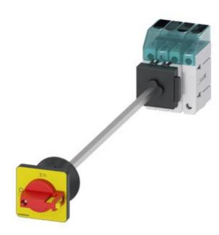
Switch disconnector 3LD3, main switch 3-polig + N, lu 63A operational switch at AC-23 A at 400 V 22,0 kW floor mounting Base mounting with door coupling center-hole 22,5 mm knob-operated mechanism red/yellow 48 x 48 mm
