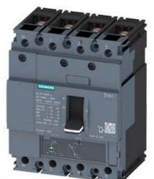
CIRCUIT BREAKER 3VA1 IEC FRAME 160 BREAKING CAPACITY CLASS S ICU=36KA @ 415 V 4-POLE, LINE PROTECTION TM220, ATFM, IN=100A OVERLOAD PROTECTION IR=70A ...100A SHORT CIRCUIT PROTECTION II=10 X IN NEUTRAL PROTECTION 100% BUSBAR CONNECTION
