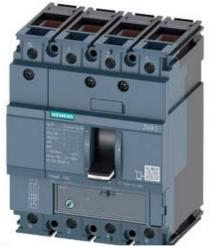
CIRCUIT BREAKER 3VA1 IEC FRAME 160 BREAKING CAPACITY CLASS H ICU=70KA @ 415 V 4-POLE, LINE PROTECTION TM220, ATFM, IN=50A OVERLOAD PROTECTION IR=35A ...50A SHORT CIRCUIT PROTECTION II=10 X IN NEUTRAL UNPROTECTED CABLE CONNECTION
