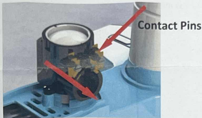
Figure 4: Unscrewing contact pins
