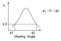
Contrast ratio K vs viewing angle ♦
