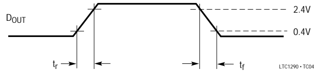
Voltage Waveform for D_{OUT} Rise and Fall Times, t_r , t_f
