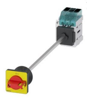
Switch disconnector 3LD3, main switch 3-polig, lu 63A operational switch at AC-23 A at 400 V 22,0 kW floor mounting Base mounting with door coupling center-hole 22,5 mm knob-operated mechanism red/yellow 48 x 48 mm with auxiliary 1NO+1NC
