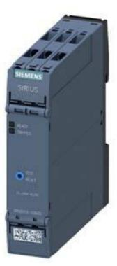
Thermistor motor prot. relay Standard evaluation unit 22.5 mm enclosure Screw terminals 2 CO contacts, hard gold-plated US = 24-240 V AC/DC Manual/Auto/Remote RESET with ATEX certification 2 LEDs (READY/TRIPPED) Protective separation Test/Reset button Open-circuit monitoring Short-circuit monitoring Non-volatile
