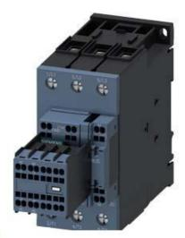
CONTACTOR,AC3:18.5KW/400V, 2NO+2NC, 48 - 80V AC/DC, WITH VARISTOR, 3-POLE, SIZE S2, SPRING-TYPE TERMINAL
