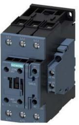
CONTACTOR,AC3:30KW/400V, 2NO+2NC, 20-33V AC/DC, WITH VARISTOR, 3-POLE, SIZE S2, SCREW TERMINAL LATERAL AUXILIARY CONTACT BLOCK
