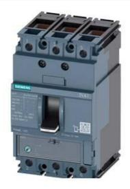
CIRCUIT BREAKER 3VA1 IEC FRAME 160 BREAKING CAPACITY CLASS M ICU=55KA @ 415 V 3-POLE, LINE PROTECTION TM220, ATFM, IN=125A OVERLOAD PROTECTION IR=87,5A ...125A SHORT CIRCUIT PROTECTION II=10 X IN CABLE CONNECTION
