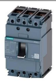
CIRCUIT BREAKER 3VA1 IEC FRAME 160 BREAKING CAPACITY CLASS S ICU=36KA @ 415 V 3-POLE, LINE PROTECTION TM210, FTFM, IN=32A OVERLOAD PROTECTION IR=32A FIXED SHORT CIRCUIT PROTECTION II=10 X IN BUSBAR CONNECTION
