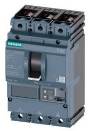
CIRCUIT BREAKER 3VA2 IEC FRAME 160 BREAKING CAPACITY CLASS H ICU=85KA @ 415 V 3POLE, LINE PROTECTION ETU550, LSI, IN=63A OVERLOAD PROTECTION IR=25A ...63A SHORT CIRCUIT PROTECTION ISD=0,6..10X IN, II=1,5..12X IN NEUTRAL PROTECTION OPTIONAL WITH EXT. CT,UPTO 160% BUSBAR CONNECTION
