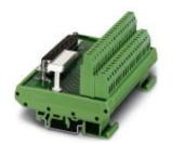
VARIOFACE module, with screw connection and D-Subminiature socket strip, for mounting on NS 35/7.5 or NS 32, 25-pos.
