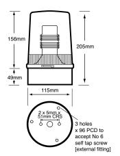
The X201/200 Series utilises a discharge capacitor and converter circuit to ignite xenon gas inside a tube, resulting in a brilliant flash of light. Xenon gas ignites virtually instantaneously so maximum brightness is obtained immediately. Xenons have an added advantage of low current consumption combined
