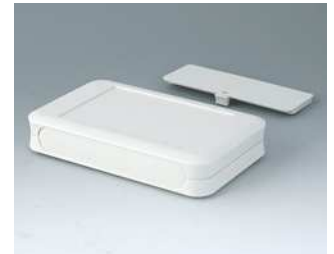
A9053117 SOFT-CASE XL ABS (UL 94 HB) grauweiß RAL 9002 92x150x28mm IP 40
