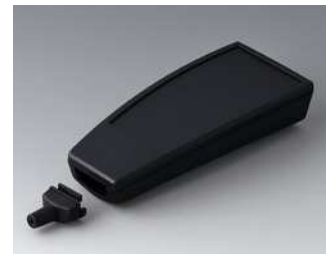
A9067349 SMART-CASE L, Ausf. V ABS (UL 94 HB) schwarz RAL 9005 140x62,7x30,5mm IP 65 opt., IP 40
