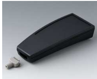
A9068149 SMART-CASE XL, Ausf. V ABS (UL 94 HB) schwarz RAL 9005 168x74,4x35,4mm IP 65 opt., IP 40
