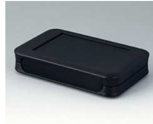
A9052209 SOFT-CASE L PMMA (IR) (UL 94 HB) schwarz RAL 9005 73x117x24mm IP 54 opt., IP 40
