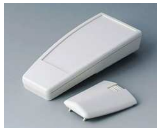
A9067107 SMART-CASE L, Ausf. I ABS (UL 94 HB) grauweiß RAL 9002 140x62,7x30,5mm IP 40
