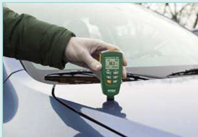
Measuring the thickness of automotive paint
