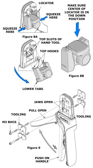
Hand Crimp Tool 1.25mm (.049") Pitch PicoBlade Receptacle Crimp Terminals
