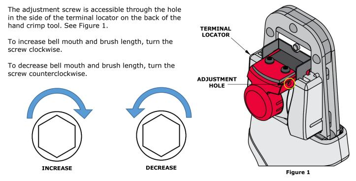
When making an adjustment, turn the adjustment screw half a rotation or less, and then re-check your bell mouth and brush length.
