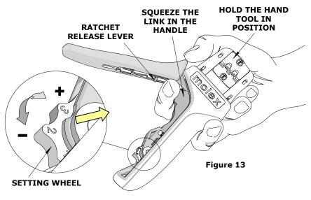
4. Check the crimp specifications or conduct a pull test after tool handle preload force is adjusted.
