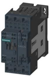
CONT. F. RAILW. A., AC-3, 11KW/400V, 1NO+1NC, AC(40-60HZ)/DC-OPERATED, UC 24V, 0,7...1,25\*US, W. VARISTOR INTEGRATED, 3-POLE SIZE S0, SPRING-TYPE TERM.
