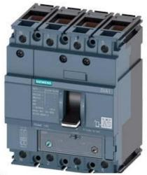
CIRCUIT BREAKER 3VA1 IEC FRAME 160 BREAKING CAPACITY CLASS S ICU=36KA @ 415 V 4-POLE, LINE PROTECTION TM240, ATAM, IN=100A OVERLOAD PROTECTION IR=70A ...100A SHORT CIRCUIT PROTECTION II=5...10 X IN NEUTRAL PROTECTION 50% CABLE CONNECTION
