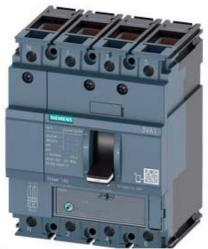
CIRCUIT BREAKER 3VA1 IEC FRAME 160 BREAKING CAPACITY CLASS N ICU=25KA @ 415 V 4-POLE, LINE PROTECTION TM220, ATFM, IN=125A OVERLOAD PROTECTION IR=87,5A ...125A SHORT CIRCUIT PROTECTION II=10 X IN NEUTRAL PROTECTION 50% CABLE CONNECTION
