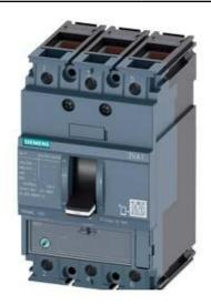
CIRCUIT BREAKER 3VA1 IEC FRAME 160 BREAKING CAPACITY CLASS S ICU=36KA @ 415 V 3-POLE, LINE PROTECTION TM220, ATFM, IN=125A OVERLOAD PROTECTION IR=87,5A ...125A SHORT CIRCUIT PROTECTION II=10 X IN CABLE CONNECTION
