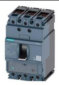
CIRCUIT BREAKER 3VA1 IEC FRAME 160 BREAKING CAPACITY CLASS S ICU=36KA @ 415 V 3-POLE, LINE PROTECTION TM240, ATAM, IN=63A OVERLOAD PROTECTION IR=44,1A ...63A SHORT CIRCUIT PROTECTION II=5...10 X IN CABLE CONNECTION
