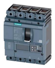
CIRCUIT BREAKER 3VA2 IEC FRAME 100 BREAKING CAPACITY CLASS C ICU=110KA @ 415 V 4POLE, LINE PROTECTION ETU850, LSI, IN=40A OVERLOAD PROTECTION IR=16A ...40A SHORT CIRCUIT PROTECTION ISD=0,6..10X IN, II=1,5..12X IN NEUTRAL PROTECTION ADJUSTABLE (OFF, UPTO 160%) CABLE CONNECTION
