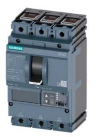
CIRCUIT BREAKER 3VA2 IEC FRAME 160 BREAKING CAPACITY CLASS C ICU=110KA @ 415 V 3POLE, LINE PROTECTION ETU860, LSIG, IN=40A OVERLOAD PROTECTION IR=16A ...40A SHORT CIRCUIT PROTECTION ISD=0,6..10X IN, II=1,5..12X IN NEUTRAL PROTECTION OPTIONAL WITH EXT. CT,UPTO 160% GROUNDFAULT, SWITCHABLE IG=0,2... 1 X IN, TG=0,050,8MS CABLE CONNECTION
