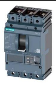
CIRCUIT BREAKER 3VA2 IEC FRAME 250 BREAKING CAPACITY CLASS C ICU=110KA @ 415 V 3POLE, LINE PROTECTION ETU860, LSIG, IN=160A OVERLOAD PROTECTION IR=64A ...160A SHORT CIRCUIT PROTECTION ISD=0,6..10X IN, II=1,5..12X IN NEUTRAL PROTECTION OPTIONAL WITH EXT. CT,UPTO 160% GROUNDFAULT, SWITCHABLE IG=0,2... 1 X IN, TG=0,050,8MS BUSBAR CONNECTION
