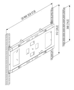
The FAU 3150 universal flat display interface is part of a modular system which enables you to create your own wall, ceiling or floor mounting solution for LCD/Plasma TV's (30-65", with VESA MIS-F, up to 70 kg). The Autolock® locking system locks the interface onto the support and prevents the display from falling of the turn and tilt unit when accidently lifted. The optional lock PFA 9008 blocks the locking system, hence preventing theft.
