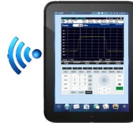
Wired/wireless\* remote control with R&S®InstrumentView PC software
