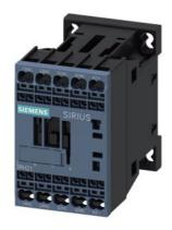
Contactor relay for railway 2 NO + 2 NC, 24-34 V DC, 0.7...1.25\*Us, with integrated varistor Size S00, Spring-type terminals suitable for PLC outputs
