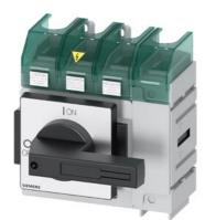
SENTRON, Molded case switch 3LD5 UL, Main switch, 4-pole, certified according to UL489 UL60947-4-1 and IEC60947-3, UL: 150A, SCCR 50kA at 480VAC, Operating power at 480VAC 3-phase: 100hp, IEC: 160A, Operating power at AC-23A at 400V: 75kW, floor mounting with direct handle, black, incl. terminal covers for the infeed side
