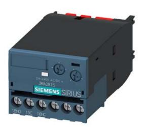
SOLID-STATE TIME-DELAY AUXILIARY SWITCH, OFF-DELAY WITHOUT AUXILIARY VOLTAGE RELAY 1 CO CONTACT 24...240V AC/DC TIME RANGE 0.05...100S FOR SNAPPING ONTO THE FRONT; FOR 3RT2 S00-S2 CONTACTORS SCREW TERMINALS INTEGRATED VARISTOR FOR DAMPING CONTACTOR COILS
