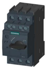
CIRCUIT-BREAKER SZ S00, FOR TRANSFORMER PROT. A-RELEASE 7...10A, N-RELEASE 208A, SCREW CONNECTION, STANDARD SW. CAPACITY W. TRANSVERSE AUX. SWITCH 1NO+1NC
