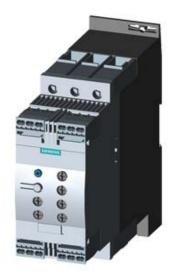
SIRIUS SOFT STARTER, S2, 63A, 37KW/500V, 40 DEGR., AC 400-600V, AC/DC 24V, SPRING-LOADED TERMINALS, THERMISTOR MOTOR PROTECTION
